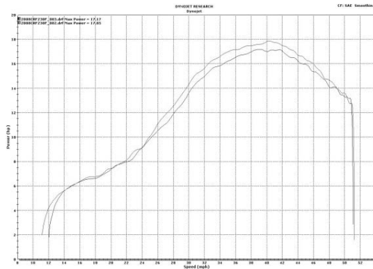
This graph shows a typical gain with a Dynojet jet kit.
