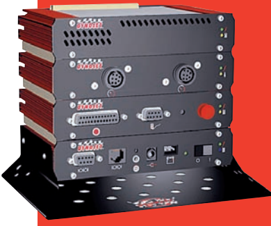
The brains behind the Dynojet was this Dynamometer EX+ hardware. The package included an atmospheric sensing module, an rpm module and a dynamometer input/output module. The CPU module contained a 32-bit processor, which acquired data from the expansion modules and communicated this data to the user-supplied computer running the WinPEP software.
